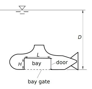
A submarine of mass *m* is submerged in water and balanced at rest so that its bottom is at depth *D*. The submarine bottom can be opened to allow access to a loading bay of length *L*, height *H*, and width *t*. From the loading bay, the submarine can be accessed through a door. The door is flush with the bay, rectangular, and measures  $H \times t$ . The bay gate is initially closed and the bay is filled with air. Knowing *H*, *t*, *D*, *L*, *m*, and water density  $\rho$ ,
