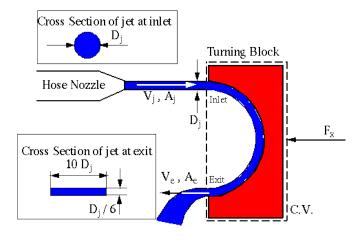
After interaction with the block, the jet turns a full 180° and flattens to an approximately rectangular cross-section (10  $D_j$  by  $D_j/6$ , as shown). Assuming the flow is steady, find
