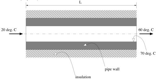
A water heater has an inlet temperature of 20° C and an outlet temperature of 60° C. The water passes through a thick-walled tube with inner and outer diameters 20 mm and 40 mm respectively. The outer wall is heavily insulated. The tube is heated electrically, with a heat generation of  $10^6$  W/m<sup>3</sup>. The heat capacity of water is 4180 J/(kg K). Calculate:
