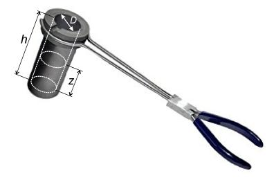
The interior cavity of a crucible is cylindrical in shape, with a diameter D = 0.125 m and a depth h = 0.125 m. Inside the crucible is molten metal with an average temperature T = 600 K. The depth of the liquid metal in the crucible is z = 0.075 m. Making the simplest assumptions about the properties of the surfaces and materials involved, estimate the rate of radiative heat loss from the surface of metal in the crucible.
