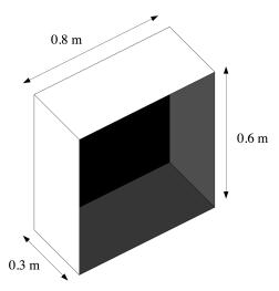
A fireplace can be modeled as an enclosure with the dimensions shown in the figure. After burning logs for a while, the walls become very hot. If their temperature is 350°C, and their emissivity is 0.7, estimate the rate of radiant heat transfer to a large room at 22°C.
