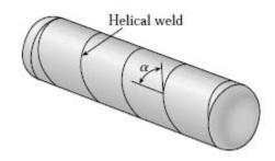
Consider a tubular shaft that transmits 100 kW at 5 Hz. The inside diameter of the shaft is to be one-third of the outside diameter. If the allowable shear stress in the shaft is 50 MPa, what is the minimum required outside diameter d?
